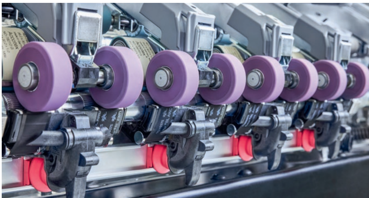
COMPACTapron guides the fibers smartly through the compacting zone and enables excellent yarn tenacity values.
